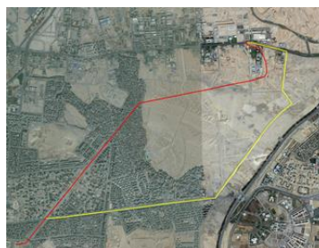
Figure (6): Map Showing the Existing High Voltage Powerlines and the Proposed Route for the Underground Cables in Ezbet El Hagana Informal Area, Nasr City, Cairo (By the Author).
