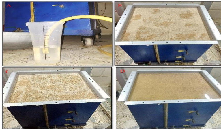
Plate 5: Measuring the rate of discharge water and stages of soil saturation.
