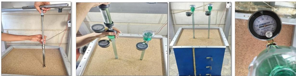
Plate 7: The stages of installing the Tensiometers and applying vacuum.
