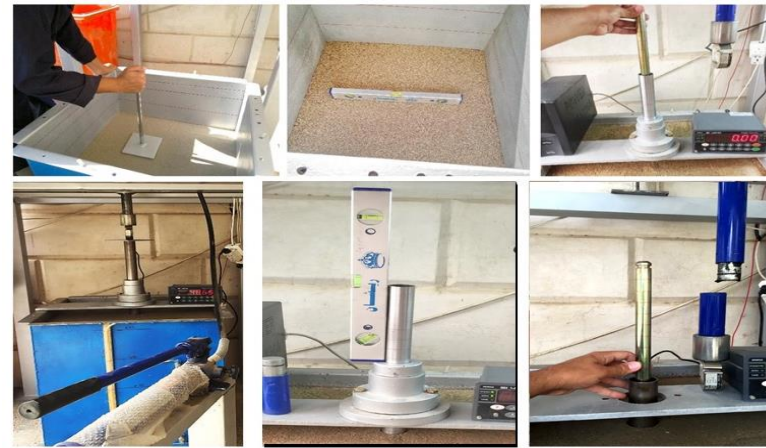
Plate 6: Preparation of soil bed and measuring the plug length.
