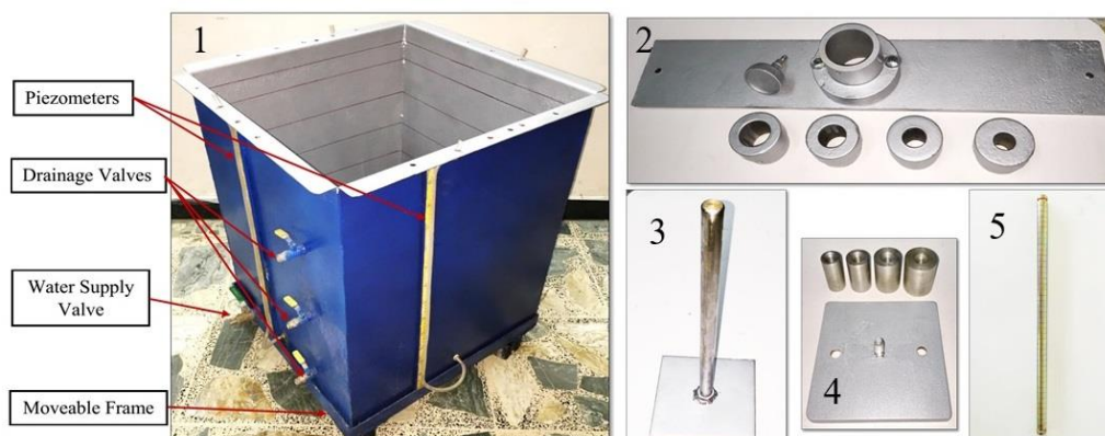
1- Steel container, 2- Pipe pile holder, 3- steel tamping hammer, 4- piles installation equipment, 5- soil plugs measurement device.
