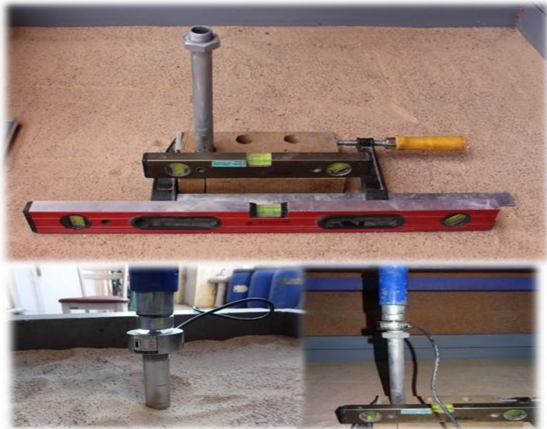
Figure (5) setting piles
