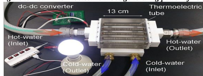
Figure .8 Four Thermoelectric tubes generating power of 10W.
