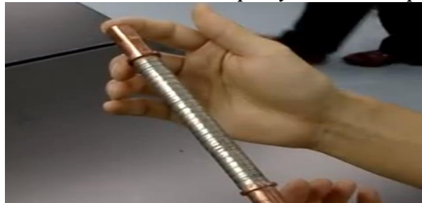
Figure.1 Thermoelectric tube developed by Panasonic Corporation
